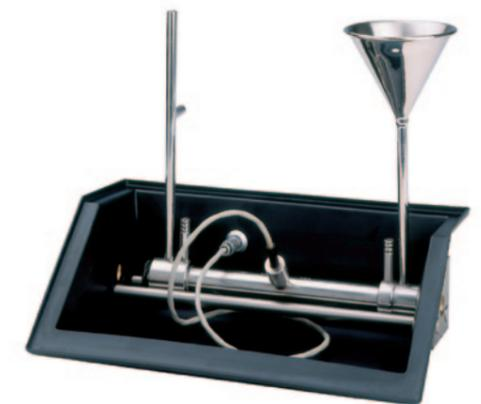
Flow-through tube with T-sensor
