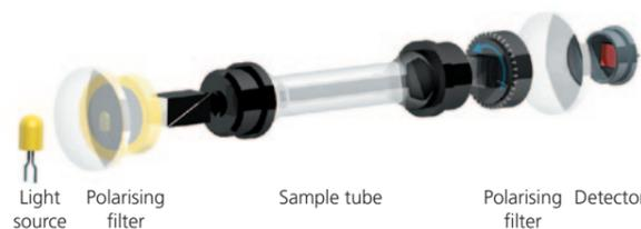
At point zero, polarizer and analyzer are set in an angle of 90° towards each other, which means that no light
