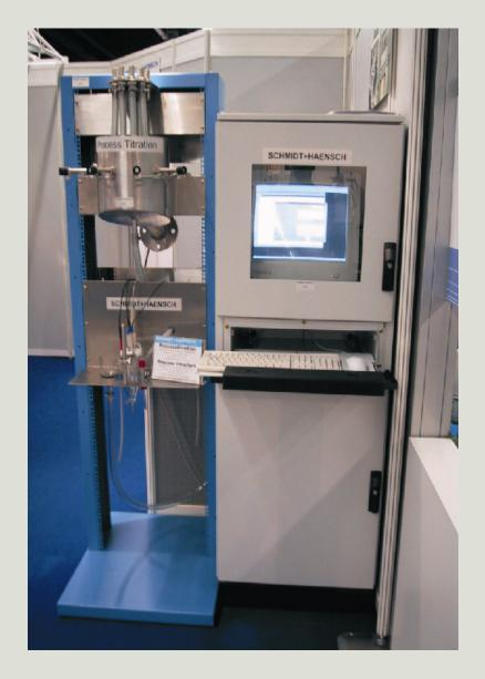
A fast and accurate analysis of important process parameters is decisive to guarantee optimal process performance. The on-line process analysis enables continuous process control in order to be able to react fast to control or regulate the process –in contrast to the time shifted and complicated laboratory determinations.
