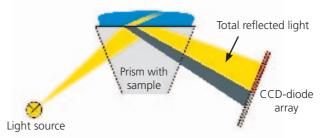
Since the light beam only probes a fraction of wavelength into the second medium very dark and turbid samples can be measured without problems. By inserting a drop of liquid on top of the measuring prism a very sharp line will appear dividing regions of below and above the critical angle. SCHMIDT+HAENSCH instruments determine the position of borderline by a high resolution CCD-diode array, thus without moving parts.
