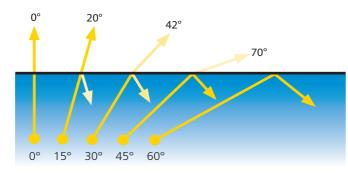
A more detailed picture below shows the case where light impinges under such special angle that the refracted beam makes an angle of 90° with the surface normal.
